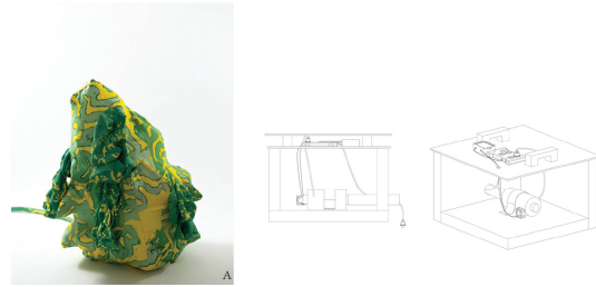
Fig 3. Thirsty For air Soft Robot. (a) Physical Sculpture. (b) Pneumonic System.
